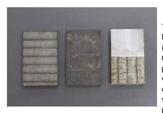
The main component of the wear-resistant layer of the low carbon steel bottom plate is high carbon and high chromium. The temperature difference between the steel plates near the welding seam is large, which will cause uneven expansion, contraction and deformation. The wear-resistant layer has high hardness and poor toughness. The coefficient of thermal
